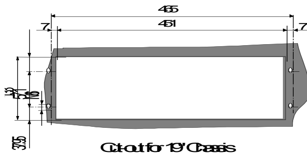
Cut-out for panel flush mounting
